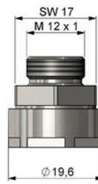
TM-TAS-CT Pivoted joint for CT sensors
