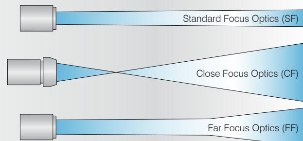
SF lenses (Standard Focus) have an almost linear relation while the CF lenses (Close Focus) have a smaller measurement spot in sensor-close distances. FF lenses (Far Focus) are especially suitable for large distances from the measurement object with a comparatively small measurement spot.
