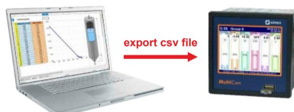
The **LookUp Table** in the user characteristics function is a great tool which allows entering individual points of the characteristics in the form of a csv file, and then importing them to any MultiCon logical channel. Additionally, the edited list may be saved, from the device level, in a new file and used to scale another channel.
