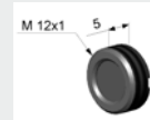
TM-CFAG-CT CF lens with external thread resp. TM-PWAG-CT Protective window with external thread
