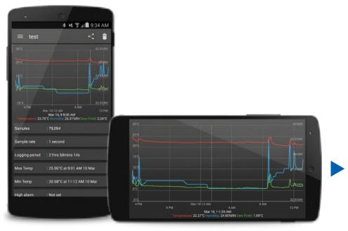
View logged temperature, humidity readings and calculated dew point, minimum and maximum values, and alarm breaches. Use zooming and panning features to view critical data with ease.
