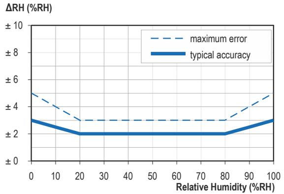
Typical accuracy of relative humidity measurements given in %RH for temperatures 0 to 80°C.
