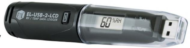
This standalone data logger measures and stores over 16,000 temperature and humidity readings from -35 to +80°C and 0 to 100%RH range at a resolution of 0.5°C and 0.5%RH.
