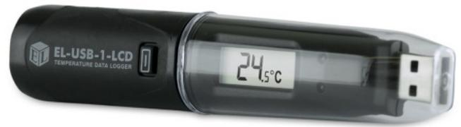
This standalone data logger measures and stores more than 16,000 temperature readings over a -35 to +80°C range with a resolution of 0.5°C.
