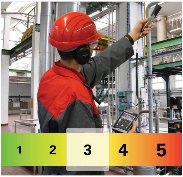
While other ultrasonic testing devices can only find leaks, **SONAPHONE** can also be used to classify their size at the same time. Based on methods of aeroacoustics **SONOTEC** developed the world's latest process for classification of leaks for the newest generation of **SONAPHONE** testing devices. The results of the patent-pending methods are plausible values for the classification of the leak size and for estimation of the savings potential.
