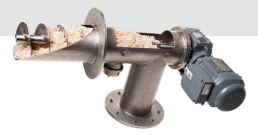
The SFM4 bypass screw compaction unit has to be placed in a free fall situation of material, e.g. in a drop shaft. A partial flow of this material is trapped in the first section of the compaction unit. The screw compactor compresses the material and conveys it into the second part of the unit, right across the installed ACO moisture sensor for the determination of the residual moisture. Then the material falls down through a drop pipe back into the process.
