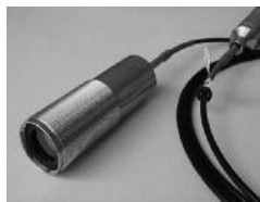
Fiber Optic connection between detector and collection optics (Lens or Lightpipe)
