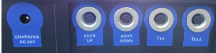
Transducers, Temperature sensor and Charging Wirings
