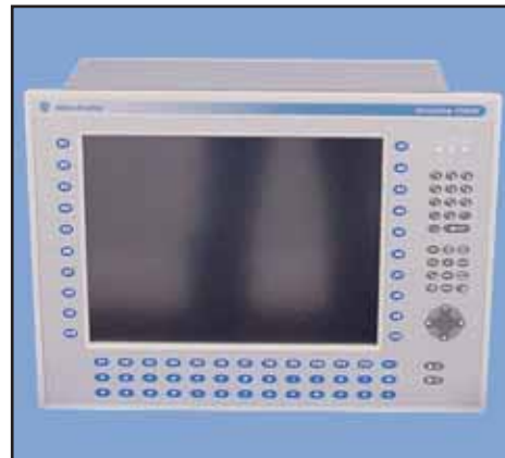
This Version of Image Processor is Recommended for Factory Floor Installation. All Buttons and Display are Sealed Against Water, Oil or Dust.
