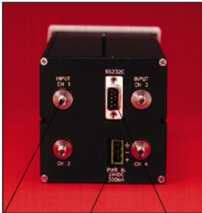
Fiber optic cable connectors (4 in total)
