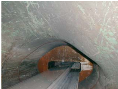
Pic. 8: Temperature control of extruded profile after the profile exits the die.
