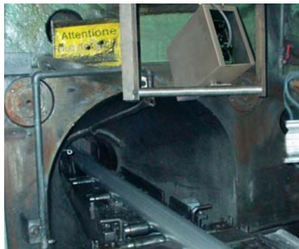
Pic. 1: Non-contact temperature measurement after the extruded profile exits the die.
